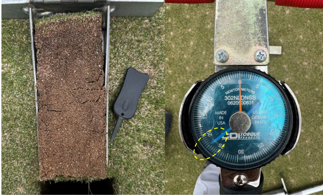
Soil profiles show deep roots (left) extending beyond 7 inches and no physical limitations to drainage. The shear strength (right) was strong at over 20 Nm.
